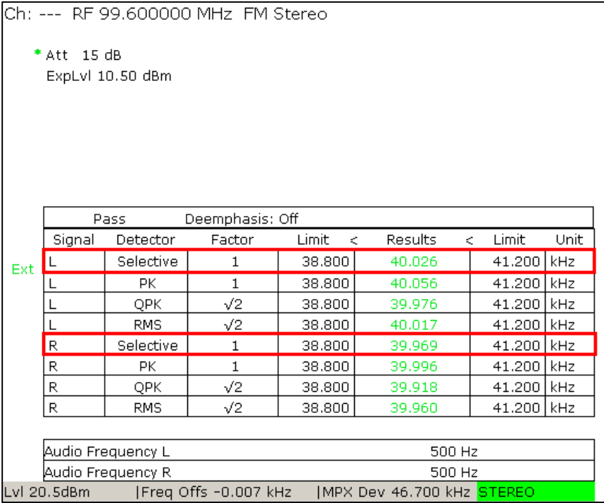
Fig. 25: "TV/Radio Analyzer/Receiver" mode, MEAS→Audio Analysis→Level: Frequency deviation for the L&R signal: Level Setup: Absolute.
