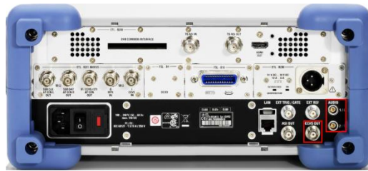
Fig. 10: The R&S®ETL has two outputs for more extensive audio analysis.
