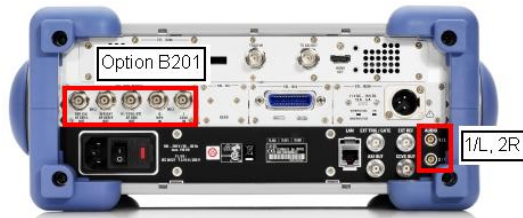
Fig. 13: Rear view of the R&S®ETL with the R&S®ETL-B201 hardware option and the 1/L, 2/R ports.
