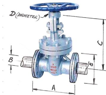
Shown in the figure above is a “gate” valve. The measurements required to manufacture a valve box for this type of valve are as follows:
