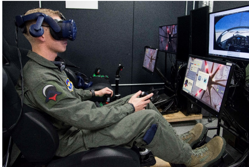
Figure 1. PTN station showing VR headset, flight controls and external displays. (U.S. Air Force photo by Sean M. Worrell)
