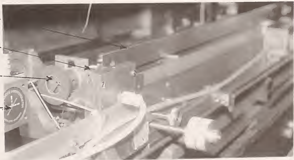
Figure 4. Schematic diagram of the NIST line scale interferometer and a photo of a long rectangular gage block mounted for measurement.
