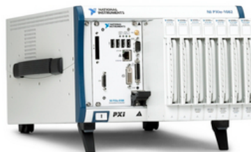
Figure 11. PXI Express Chassis with SC Express Sensor Measurement Modules
