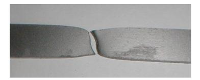
Figure 2 - Tensile specimen pulled to fracture. Depicts region where necking occurred.
