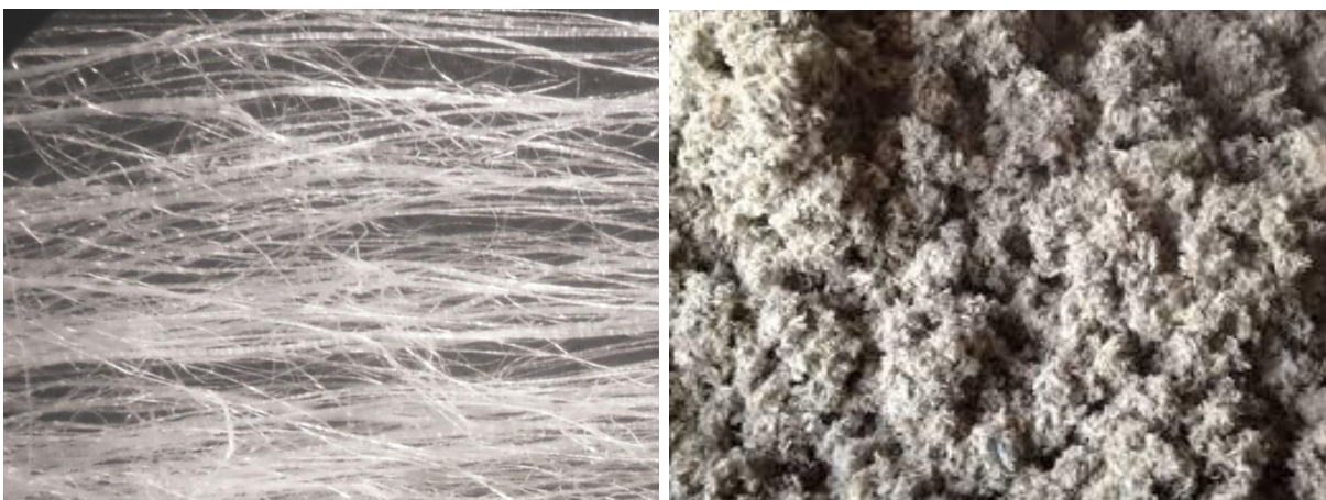
Figure 2.13: Organic fibres. Left: Hemp. Right: Cellulose
