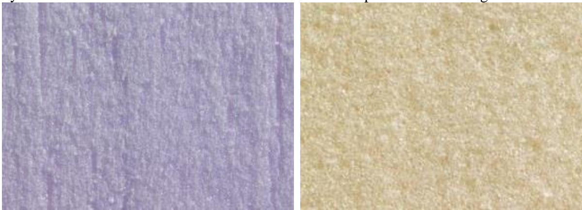
Figure 2.18: Microstructure of extruded polystyrene (left) and polyurethane foam (right). © SWISSPOR.
