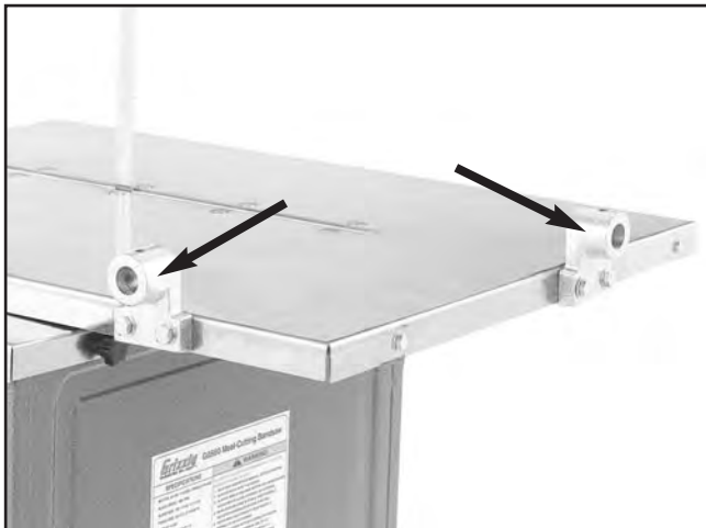
Figure 25. Fence supports to table.
