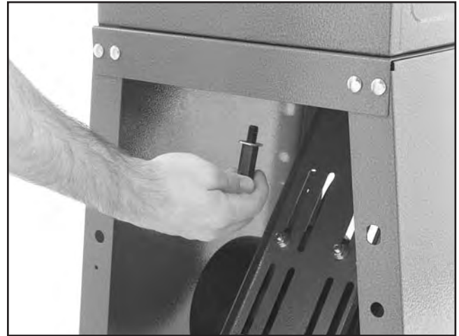
Figure 16. Installing special hex bolt.
