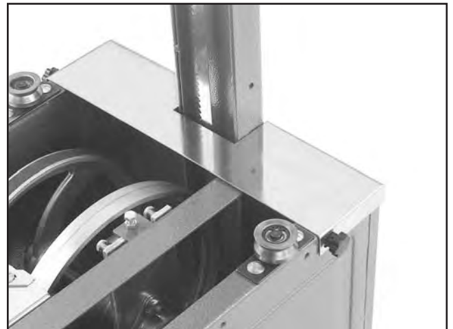
Figure 19. Table guard installed.
