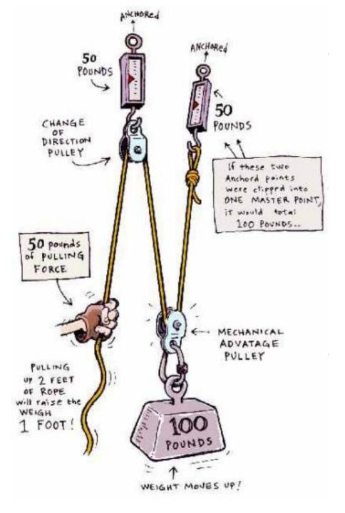
A machine's ideal mechanical advantage is its mechanical advantage with 100% efficiency.
