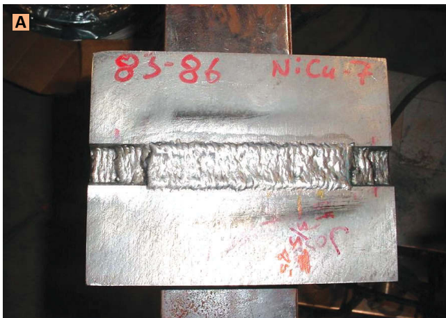
Fig. 3 — A — General view of Ti-clad steel welded joints made with the CSC-GMAW process; B — joint made with a combination of the CSC-GMAW and the GTAW-P processes.
