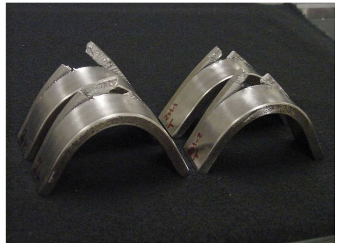
Fig. 8 — General view of side bend samples obtained from NiCu-Ti welded joints in the as-welded and PWHT conditions (CSC-GMAW process).
