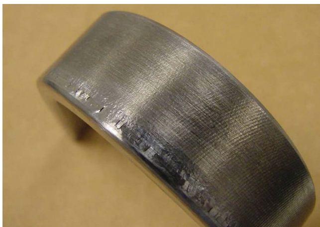
Fig. 9 — Cracks observed in longitudinal side bend samples obtained from Ti-V-Fe welded joints in the PWHT condition (GTAW-P process).
