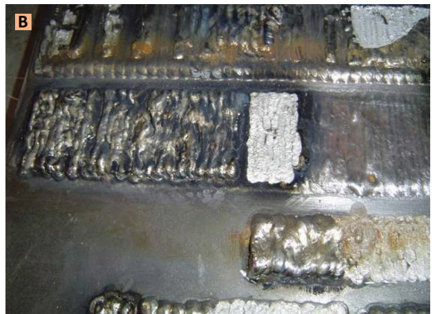
Fig. 1 — A — Titanium deposit layer that cracked and broke off a commercially pure Fe weld deposit during cooling; B — weld deposit that cracked.
