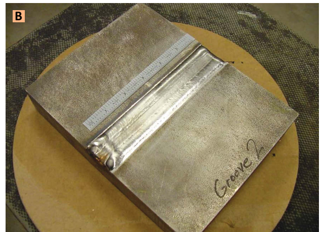
Fig. 3 — A — General view of Ti-clad steel welded joints made with the CSC-GMAW process; B — joint made with a combination of the CSC-GMAW and the GTAW-P processes.
