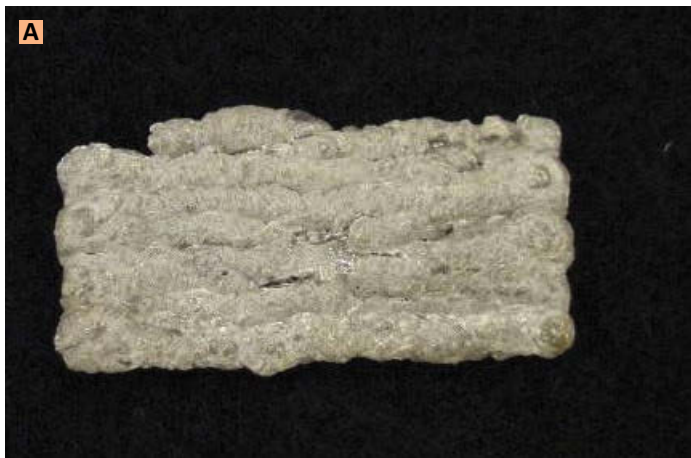
Fig. 1 — A — Titanium deposit layer that cracked and broke off a commercially pure Fe weld deposit during cooling; B — weld deposit that cracked.
