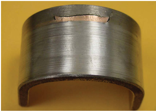
Fig. 11 — General view of side bend samples obtained from Cu-Ti welded joints in the as-welded and PWHT conditions (CSC-GMAW process).
