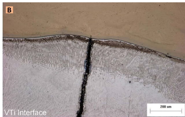
Fig. 10 — A — Microcracking observed in the Fe-V interface of welded joints deposited with the GTAW-P process; B — crack arrested at the V-Ti interface.
