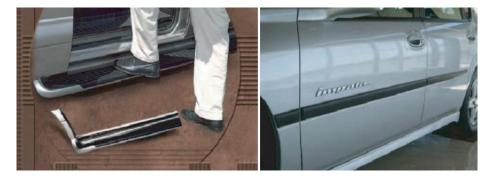
**Figure 8**: M-Van step Assist: 1 st commercial launch for TPO nano-composite application [66]
