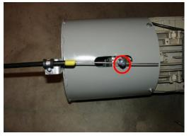
Place exposed end of brake release cable through the thru-hole on brake release arm.
