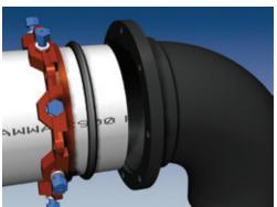
Identify the pipe. The 2000PV is for use with PVC and HDPE pipe. The 4 inch through 12 inch size may be used on C900, IPS, and C909 PVC pipe as well as C906 HDPE pipe. Check to see if the spacers under the screws are in place. If the pipe is C900 or is ductile iron O.D., proceed with spacers in place. If the pipe is IPS O.D., remove the spacers. Since 3 inch and 14 inch through 24 inch restraints are only used with one pipe diameter, no spacers are used.
