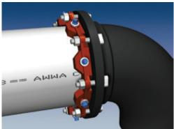
If removal is necessary, utilize the 5% inch hex heads provided. If reassembly is required, assemble the joint in the same manner as above; tighten the screws to 60 to 80 ft-lbs. If the Series 2000PV restraint is removed from the pipe, be sure that all of the screws, spacers (if required), and wedges are in place before the restraint is reassembled.
