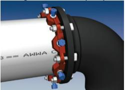
Tighten the torque limiting twist-off nuts in a clockwise direction (direction indicated by arrow on top of nut) until all wedges are in firm contact with the pipe surface. Continue tightening in an alternating manner until all of the nuts have been twisted off.
