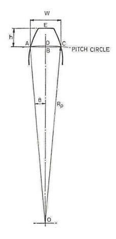
Fig.7.3. Measurement of tooth thickness at pitch circle diameter **2. Measurement of tooth width/thickness at Constant Chord**
