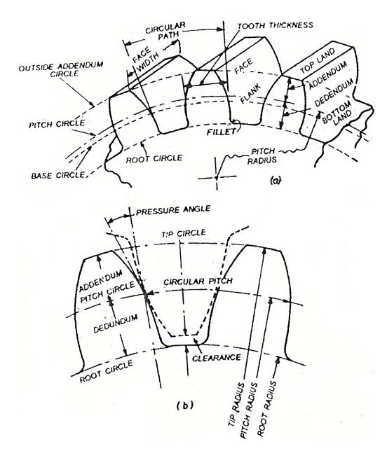
Fig.7.2. Spur gear tooth gear
