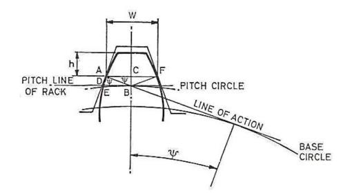
Fig.7.4. Measurement of tooth thickness at constant chord
