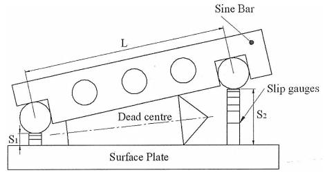
Fig.6.1. Experimental setup to measure taper angle using Sine bar
