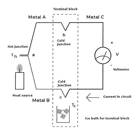
Fig. 2.1 Temperature measuring circuit using Thermocouple
