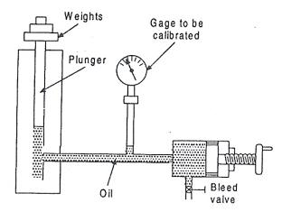
Fig4.2. Dead weight pressure gauge
