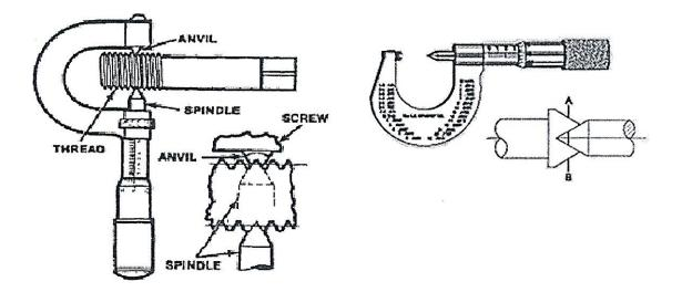
Fig.11.3. Screw thread micrometer
