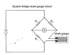
Fig.l.l c. Quarter bridge connection
