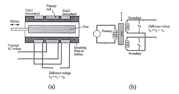
Fig.3.1. Schematic diagram of LVDT
