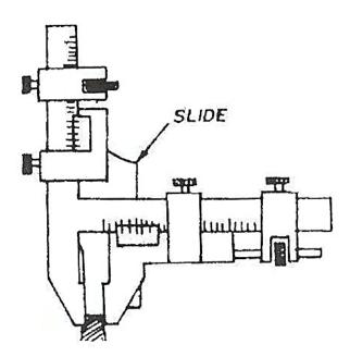
Fig. 7.1. Gear tooth vernier caliper
