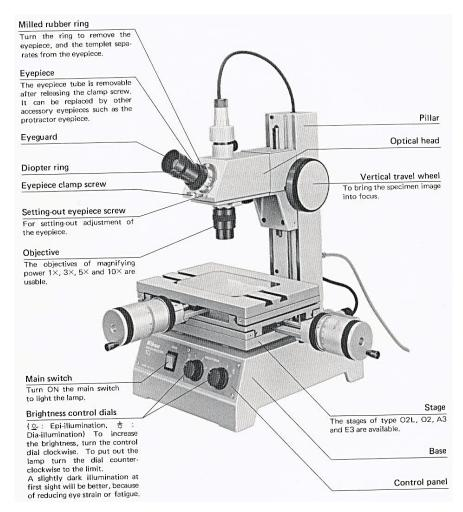
Fig.9.1 Tool maker's microscope (Measuroscope)
