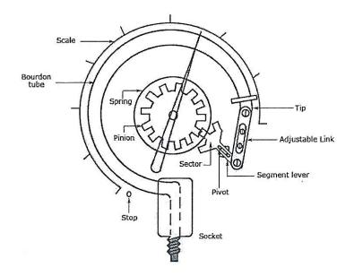
Fig 4.1. Bourdon tube pressure gauge
