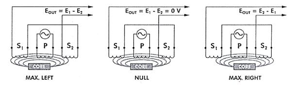
Fig.3.2. Three different cases of LVDT core position
