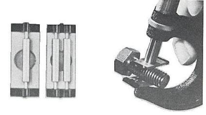
Fig.11.1. Set-up for measuring effective diameter using three
