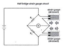
Fig.l.l d. half bridge connection
