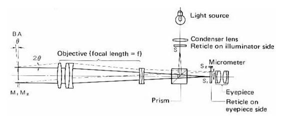
Fig.10.1. Working principle of Autocollimator
