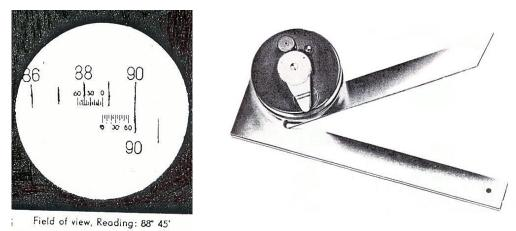
Fig.6.2. Optical bevel protractor
