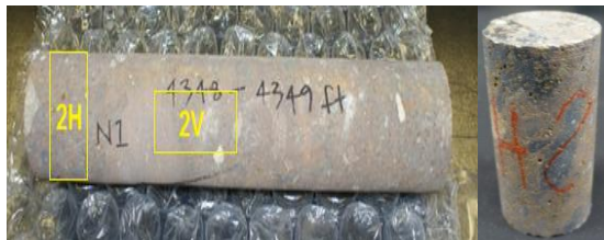
Figure 4: drilled core N1 from 4348-4349 feet depth showing the location of the plugs; Core plug of N1-4348-2H before triaxial tests.
