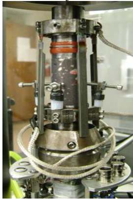
Figure 14: sample (fractured tuff) assemble ready for multistage triaxial joint shear test.
