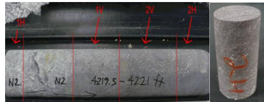
Figure 6: drilled core N2 from 4219 feet depth showing the location of the plugs; Core plug of N2-4219-2H before triaxial tests.
