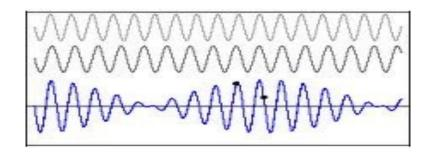
Waves alternate between "in phase" and "out of phase"
