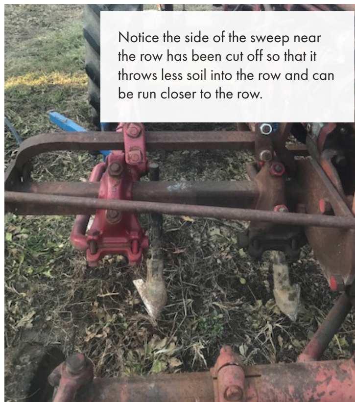
fig. 9: sweeps on an older American cultivator.
