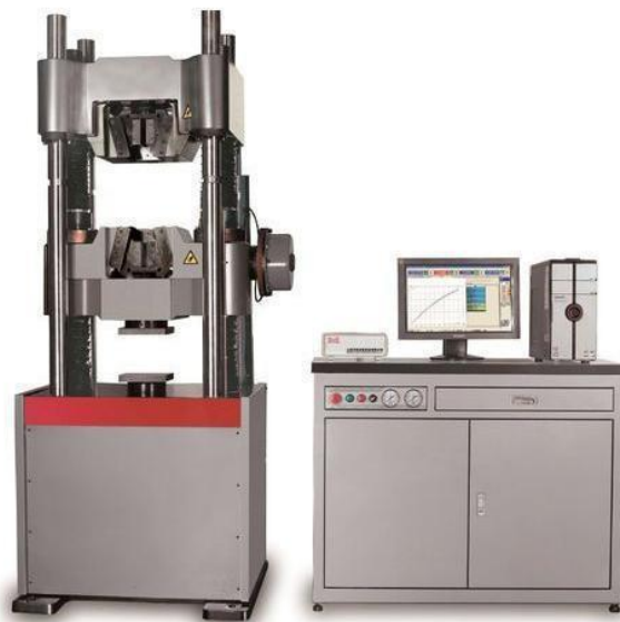
Figure 14-1: Universal Testing Machine for different beams
