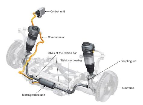
FIGURE 3 eARC system components and their installation in a front axle configuration for an Audi AQ7 (© Audi, Schaeffler)
