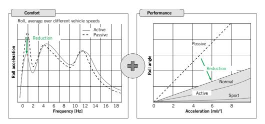
FIGURE 2 Qualitative presentation of reductions in roll accelerations and roll angles due to the eARC system for increase in comfort (left) and performance (right) [2] (© Porsche)
