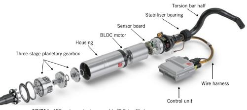
FIGURE 4 eARC system actuator assembly (© Schaeffler)
