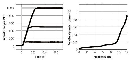
FIGURE 6 Step response of the actuator torque (left) and relative dynamic rigidity of the actuator (right) (© Schaeffler)
