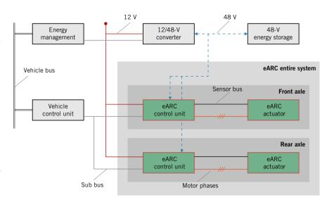
FIGURE 1 Control unit topology and connecting of the eARC entire system to the vehicle architecture (© Schaeffler)
