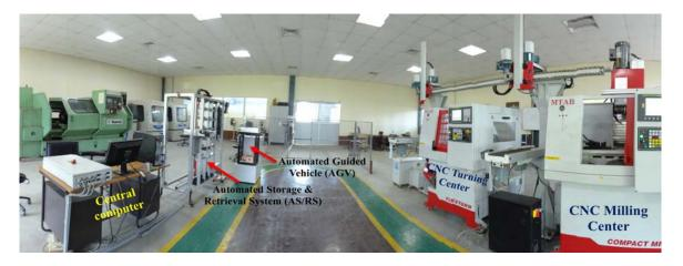
Figure 1.2.4 A FMS Setup
