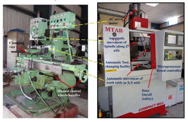
Figure 1.2.1 Comparison between a conventional machine tool and a CNC machine tool
