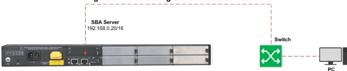
Figure 8-4: Connecting OSN3 Module to Network
