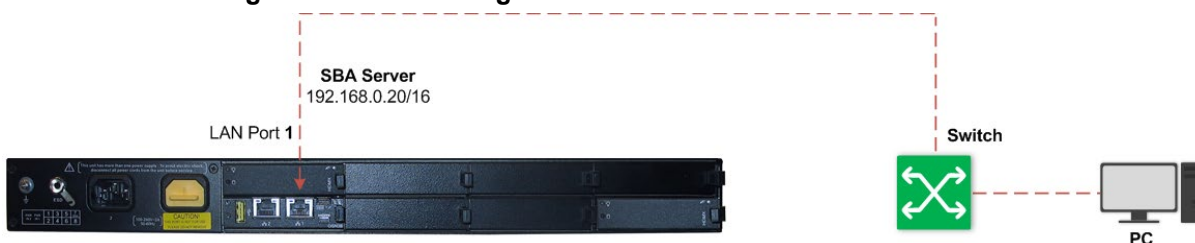
Figure 8-3: Connecting OSN3B and OSN4 Module to Network
