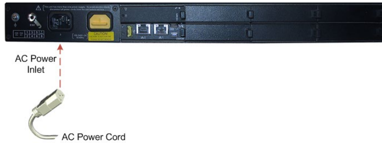
Figure 8-5: Powering on Device
