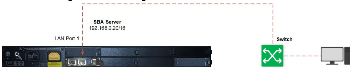
Figure 8-2: Connecting OSN3C and OSN4B Module to Network
