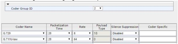
The procedure below describes how to configure an Allowed Coders Group to ensure that voice sent to the Windstream SIP Trunk uses the G.729 coder whenever possible. Note that this Allowed Coders Group ID was assigned to the IP Profile belonging to the Windstream SIP Trunk in the previous step (see Section 4.6 on page 48).
