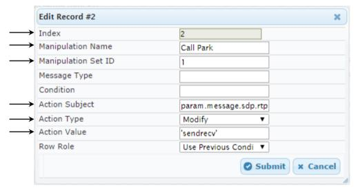
5. The following rule attempts to normalize the call processing state back to Lync 2013 for the correct reply to the initially received "sendonly". For every SIP Re-INVITE message with the variable set to '1', change RTP mode to "recvonly". This SIP Re-INVITE message is the response sent from the Windstream SIP Trunk to the Lync initiated Hold.
