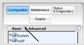
Note that when the E-SBC is reset, the Navigation tree reverts to Basic-menu display.
