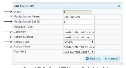
Figure 4-55: Configured SIP Message Manipulation Rules
