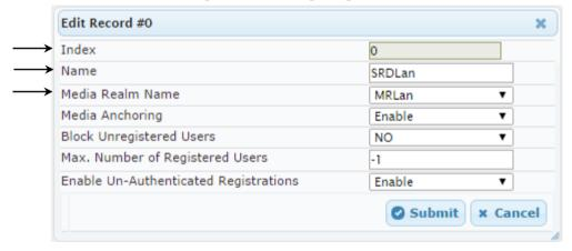
Configure an SRD for the E-SBC's external interface (toward the Windstream SIP Trunk):
