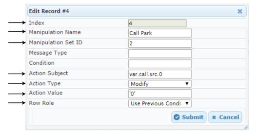
7. Configure another manipulation rule (Manipulation Set 4) for Windstream SIP Trunk. This rule applies to messages sent to the Windstream SIP Trunk (IP Group 2) in call forward scenario. This replaces the user part of the From Header with the value from History Info Header.
