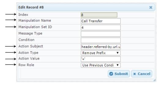
11. Configure another manipulation rule (Manipulation Set 4) for Windstream SIP Trunk. This rule applies to messages sent to the Windstream SIP Trunk (IP Group 2). This rule replaces the **user** part of the **From** Header with the value from Referred-By Header.
