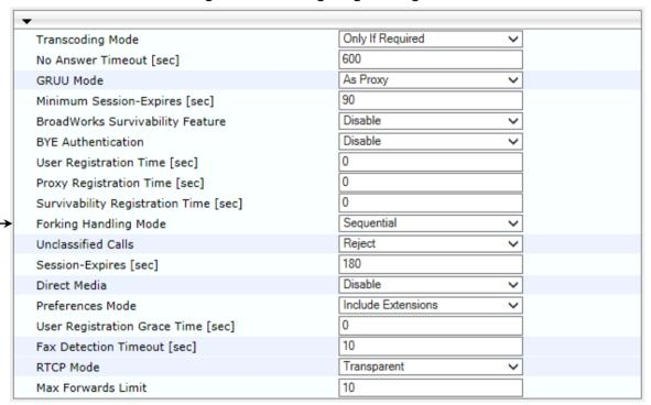
Figure 4-59: Configuring Forking Mode
