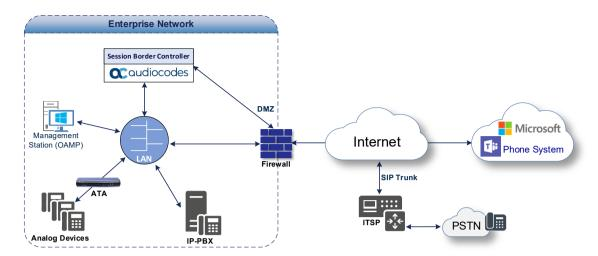
Figure 2-2: Connection Topology with SIP Trunk on the WAN
