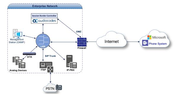
Figure 2-1: Connection Topology with SIP Trunk on the LAN
