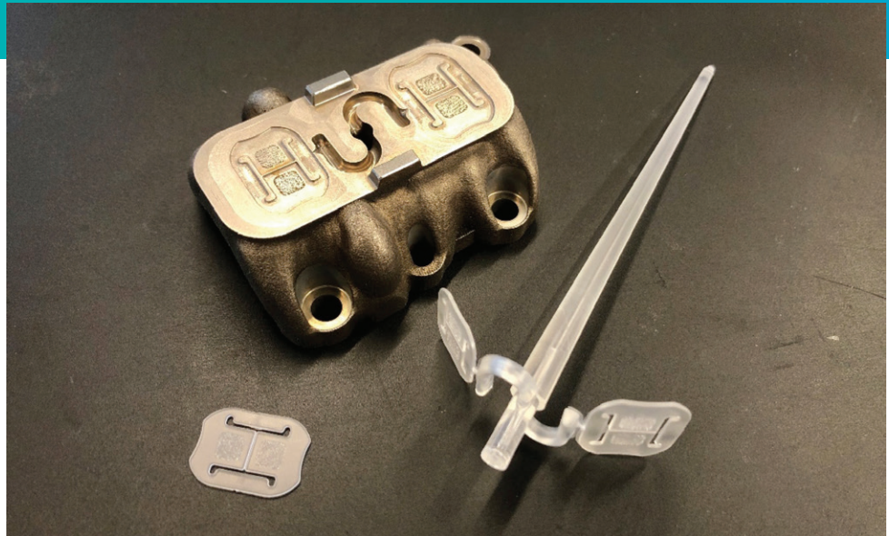
Figure 6. The final mold and its plastic part.
