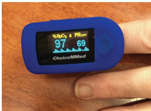
Pulse oximeter showing oxygen saturation, heart rate and wave form (showing heart rhythm)
