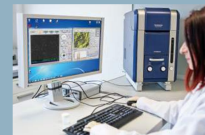
Surface analyses via electronic scanning microscopy (SEM) and determination of elements (EDX)
