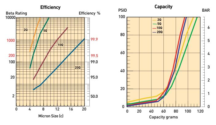
Results typical from Multi-pass tests run per test standard ISO 16889 @ 50 gpm to 100 psid terminal - 10 mg/L BUGL Refer to Appendix on pages 227-228 for relationship to test standard ISO 4572.
