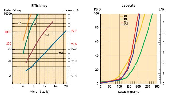
Results typical from Multi-pass tests run per test standard ISO 16889 @ 80 gpm to 100 psid terminal - 10 mg/L BUGL Refer to Appendix on pages 227-228 for relationship to test standard ISO 4572.
