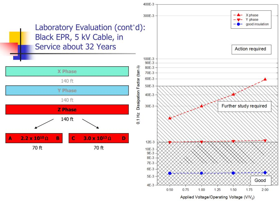
Laboratory Evaluation (cont'd): Black EPR, 5 kV Cable, in Service about 32 Years
