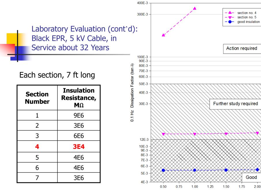
Applied Voltage/Operating Voltage (V/V<sub>0</sub>)
