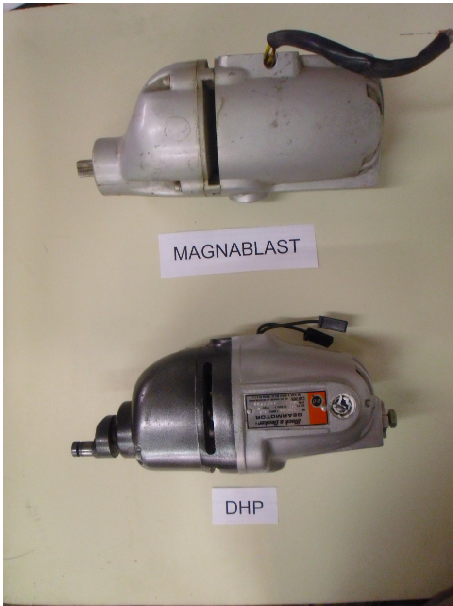
Figure 3-2 typical circuit breaker charging motor
