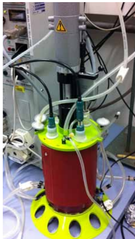
Gymetrics' wireless, battery-less temperature and pH sensor for cell culture measurement.
