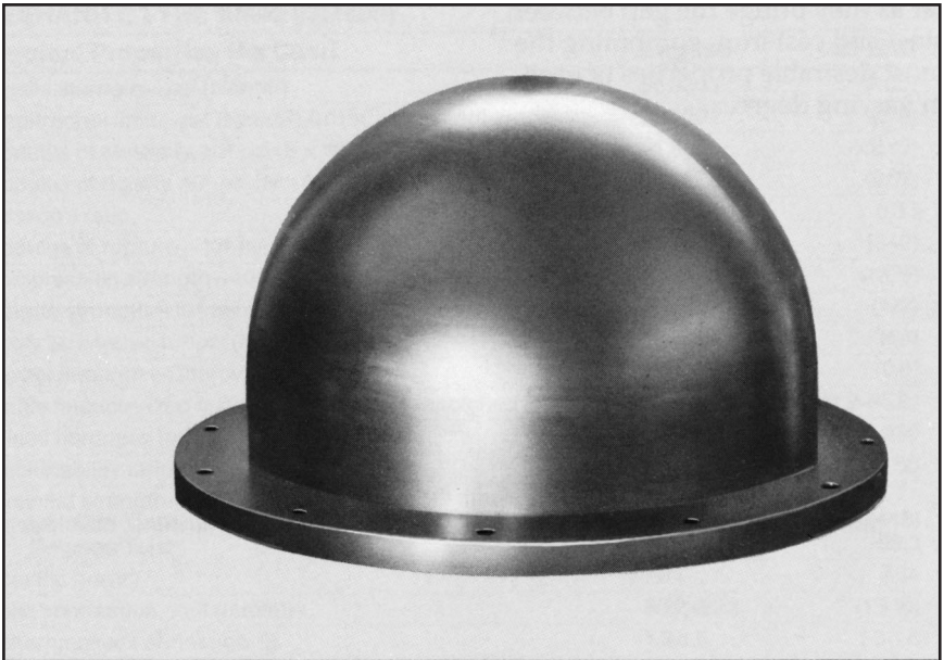
This 6680 lb. Meehanite mandrel was cast in type SH 100. Machined "as cast." Hardened to 430-500 Brinell and then ground to size.
