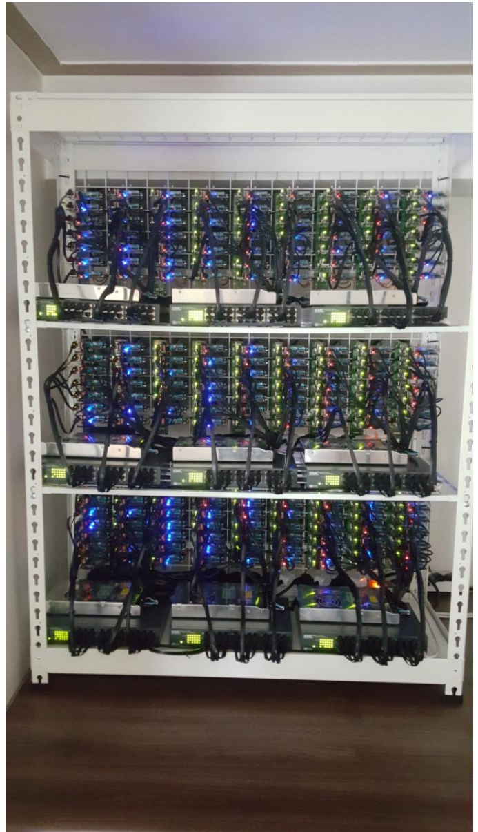
Hardkernel spent several days building this big cluster computer using 200 ODROID-MC1 units with 1600 CPU cores and 400GB RAM
