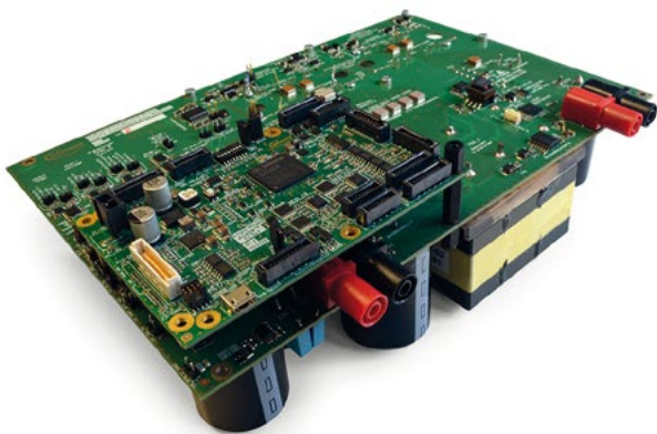
Figure 9: LLC prototype top side (left) and bottom side (right) showing CoolMOS™ CFD7A Easy1B press-fit power modules.
