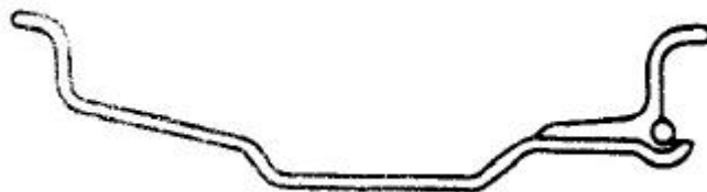
Gambar 8. Semi Drop Center Rim
