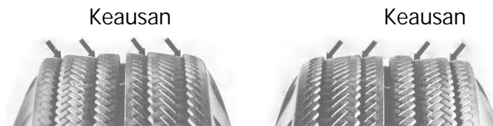
Gambar 31. Keausan Ban Akibat Toe – out
