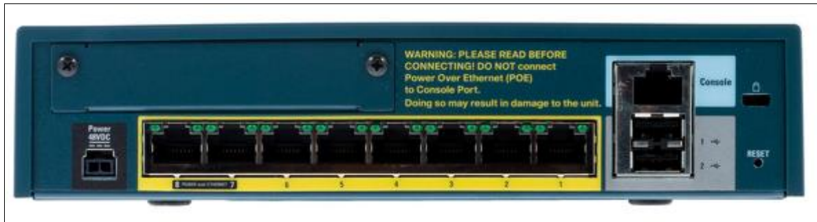
Figura 20: Controlador Wireless Cisco AIR-WLC2125-K9 (Costas)
