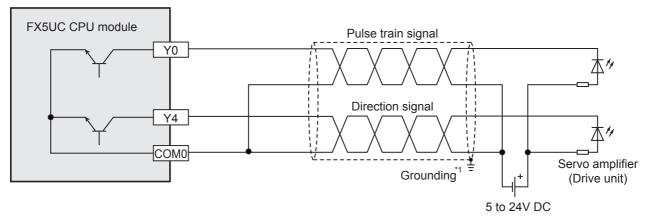
\*1 To ground the unit, refer to the servo amplifier (drive unit) manual. If the grounding method is not specified, carry out class-D grounding. 2
