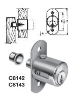
APPLICATION - C8140 is for sliding glass doors. C8142 and C8143 are for wood sliding doors and require a 7/8" dia. hole in front door for cylinder. C8150 is used internally on filing cabinets to gang lock drawers.
