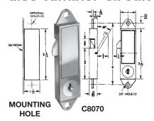
**APPLICATION** – For right handed metal doors of electrical circuit breaker cabinets. **OPERATION** – Key removable in both locked and unlocked positions. Push plate operates spring bolt. Unlocked, push plate acts as spring latch.
