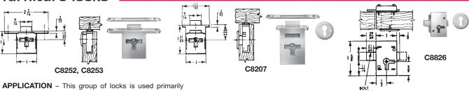
on furniture and other fine cabinetry. C8826 is surface mounted and requires hole for key entry, all other locks require full 11/32" x depth of lock. Additional mortising, required for lock selvedge plus hole for key entry.
