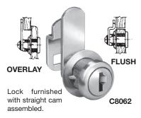
APPLICATION - For drawers, R.H. or L.H. doors with overlay (straight cam) or flush (formed cam) construction. For overlay application, the combined thickness of front and frame cannot exceed the 7/8" cylinder length. See above for mounting hole detail.
