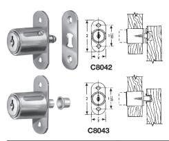
APPLICATION - For wood sliding doors. Requires a 7/8" dia. hole in front door for cylinder.
