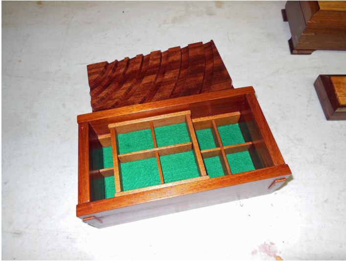
Bob McElfresh: Jewelry Box Mahogany box with bubinga top Design from wood magazine
