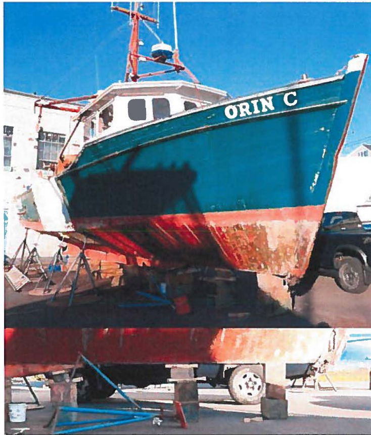
Photo from FisherlyNation.com article showing keel damage
