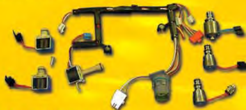
MS 4L60E H ▲ Fits 4L60E '93-95 With Solenoids and Internal Wiring Harness. Warning will not work in '96-Up Vehicles. * Internal harness may be purchased separately.
