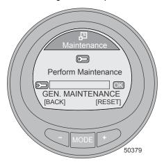
A window will pop up asking HAS SCHEDULED MAINTENANCE BEEN PERFORMED? Press the "+" button—NO, to return to the Maintenance screen, or press the "-" button—YES, to reset the scheduled maintenance screen.
