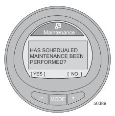
6. After pressing the "-" button—YES, to reset the scheduled maintenance screen, the bar graph will reset to 100 hours. Press the "-" button to exit the Maintenance window and return to the Main Menu, or press NEXT to exit the maintenance screen to the next full screen, or press MENU to repeat the scheduled maintenance reset process.
