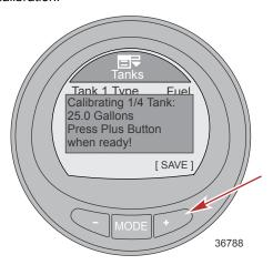
19. The fuel level sensor must change a minimal value when adding fuel. If the fuel level sensor does not change to the minimal value any time during the add fuel calibration, an error message stating the calibration is defaulting to values—Error! Defaulting to values... will be visible on the screen. The manual calibration process will stop when the error message appears. The fuel tank must be emptied and the manual calibration process must be repeated.
