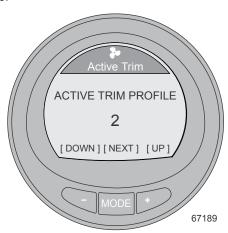
After selecting an Active Trim profile, pressing the MODE button will take the operator to the next propulsion screen. The Active Trim status will remain enabled until the Active Trim feature is disabled, by pressing the "-" button ("OFF").
