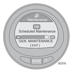
4. If the bar graph is not visible, the engine scheduled maintenance has passed 100 hours and the screen will change to Perform Maintenance. Press the "+" button to begin the reset procedure.
