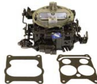
18-7613-1 CARBURETOR 4 Barrel - Carter (Weber) Replaces: 3310-806969A1, 3310-806969R01 (Remanufactured)
