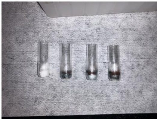
Figure 12: Blank, 0.1 g, 0.3 g, and 0.5 g copper columns
