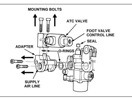
ATC Valve Replacement (ABS Valve Package) (Cont.)
