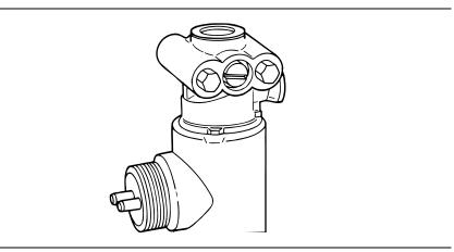
**ATC Valve Solenoid Pins**
