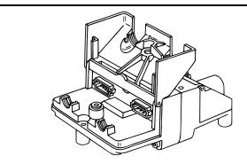
D Version Frame-Mounted ECU Connector Ports
