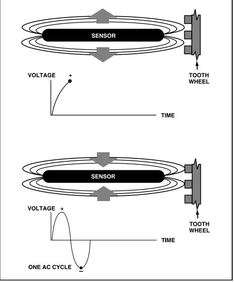
**Magnetic Pickup-Type Sensor Operation**
