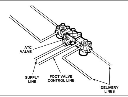
ABS Valve Package with ATC Valve
