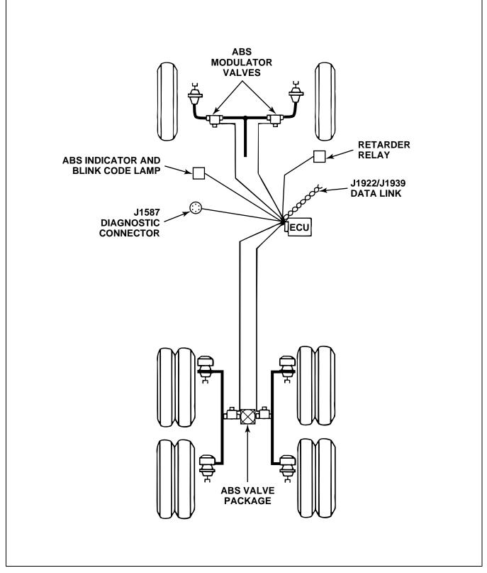
**ABS/ATC Processing and Output Components**
