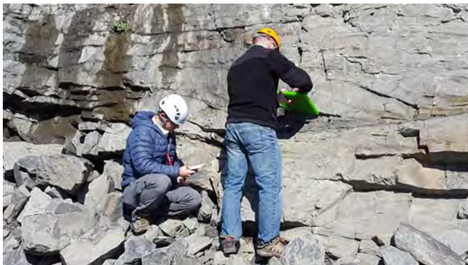
Darrin Burton (Affiliated Faculty) and Andrew Reisdorf (MS Student) work the outcrops of the Middle Atoka in Webo Quarry Arkansas, building a database to condition a reservoir model of this complex prograding deltaic body.
