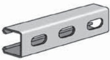
AS 500EH SS/ZTC/HG Channel with Elongated Holes Size: 1 5 / 8 " x 1 3 / 16 " x 14 GA. 9 / 16 " x 1 1 / 8 " Elongated Holes on 2" Centers. Page 81
