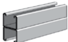
AS 200EH BTB Welded Channel Size: 1 5 / 8 " x 3 1 / 4 " x 12 GA. Two Pcs. AS 200EH Welded Back-to-Back. 9 1 / 16 " x 1 1 / 8 " Elongated Holes on 2" Centers. Page 24
