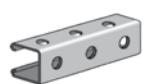
AS 200H3 Channel with Holes on all Three Sides Size: 1 5 / 8 " x 1 5 / 8 " x 12 GA. 9 1 / 16 " Holes on all three sides are on 1 7 / 8 " Centers. Page 23
