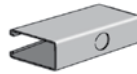
AS 100KO Channel with Knock Outs Size: 1 5 / 8 " x 3 1 / 4 " x 12 GA. 7 1 / 8 " Knock Outs on 6" Centers. Page 19
