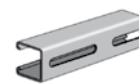
AS 200S Channel with Long Slots Size: 1 5 / 8 " x 1 5 / 8 " x 12 GA. 1 3 / 32 " x 3" Slots on 4" Centers. Page 23
