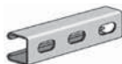
AS 500EH Channel with Elongated Holes Size: 1 5 / 8 " x 1 3 / 16 " x 14 GA. 9/16" x 1 1 / 8 " Elongated Holes on 2" Centers. Page 32
