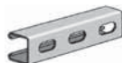
AS 520EH Channel with Elongated Holes Size: 1 5 / 8 " x 1 3 / 16 " x 12 GA. 9/16" x 1 1 / 8 " Elongated Holes on 2" Centers. Page 34
