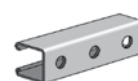
AS 210H Channel with Holes Size: 1 5 / 8 " x 1 5 / 8 " x 14 GA. 9 1 / 16 " Holes on 1 7 / 8 " Centers. Page 26
