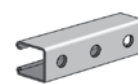
AS 200H Channel with Holes Size: 1 5 / 8 " x 1 5 / 8 " x 12 GA. 9 1 / 16 " Holes on 1 7 / 8 " Centers. Page 23
