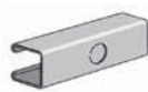
AS 300KO Channel with Knock Outs Size: 1 5 / 8 " x 1 3 / 8 " x 12 GA. 7/8" Knock Outs on 6" Centers. Page 28
