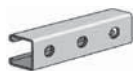
AS 500H Channel with Holes Size: 1 5 / 8 " x 1 3 / 16 " x 14 GA. 9/16" Holes on 1 7 / 8 " Centers. Page 32
