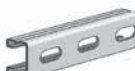
AS 560EH Channel with Elongated Holes Size: 1 5 / 8 " x 1 3 / 16 " x 16 GA. 9/16" x 1 1 / 8 " Elongated Holes on 2" Centers. Page 36
