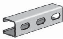
AS 200EH SS/ZTC/HG Channel with Elongated Holes Size: 1 5 / 8 " x 1 5 / 8 " x 12 GA. 9 / 16 " x 1 1 / 8 " Elongated Holes on 2" Centers. Page 77
