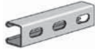
AS 400EH Channel with Elongated Holes Size: 1 5 / 8 " x 1" x 12 GA. 9/16" x 1 1 / 8 " Elongated Holes on 2" Centers. Page 30
