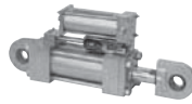
Fig. 200 & C-200 / Fig. 201 & C-201 Hydraulic Shock & Sway Suppressor (Snubber) Size Range: Nine standard sizes with cylinder bores of 1 1/2" to 8" with normal load ratings from 3,000 (LBS) to 128,000 (LBS). All are available with 5", 10", 15" or 20" strokes except the 1 1/2" size which is offered with 5" and 10" strokes only. Snubbers are available with integral or remote reservoirs.
