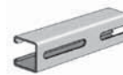
AS 300S Channel with Long Slots Size: 1 5 / 8 " x 1 3 / 8 " x 12 GA. 1 3 / 32 " x 3" Slots on 4" Centers. Page 28
