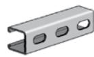
AS 200EH Channel with Elongated Holes Size: 1 5 / 8 " x 1 5 / 8 " x 12 GA. 9 1 / 16 " x 1 1 / 8 " Elongated Holes on 2" Centers. Page 23
