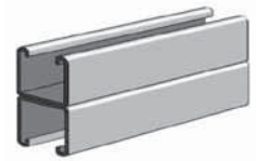
AS 200EH BTB SS/ZTC/HG Welded Channel Size: 1 5 / 8 " x 3 1 / 4 " x 12 GA. Two Pcs. AS 200EH Welded Back-to-Back. 9 / 16 " x 1 1 / 8 " Elongated Holes on 2" Centers Page 77
