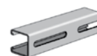
AS 210S Channel with Long Slots Size: 1 5 / 8 " x 1 5 / 8 " x 14 GA. 1 3 / 32 " x 3" Slots on 4" Centers. Page 26
