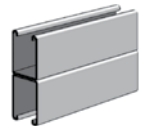
AS 150BTB Welded Channel Size: 1 5 / 8 " x 4 7 / 8 " x 12 GA. Two Pcs. AS 150 Welded Back-to-Back. Pages 20 & 21
