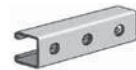
AS 400H Channel with Holes Size: 1 5 / 8 " x 1" x 12 GA. 9/16" Holes on 1 7 / 8 " Centers. Page 30
