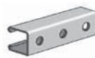
AS 300H Channel with Holes Size: 1 5 / 8 " x 1 3 / 8 " x 12 GA. 9/16" Holes on 1 7 / 8 " Centers. Page 28
