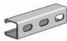
AS 300EH Channel with Elongated Holes Size: 1 5 / 8 " x 1 3 / 8 " x 12 GA. 9/16" x 1 1 / 8 " Elongated Holes on 2" Centers. Page 28
