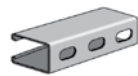
AS 150EH Channel with Elongated Holes Size: 1 5 / 8 " x 2 7 / 16 " x 12 GA. 9 1 / 16 " x 1 1 / 8 " Elongated Holes on 2" Centers. Page 21
