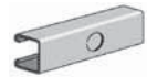
AS 400KO Channel with Knock Outs Size: 1 5 / 8 " x 1" x 12 GA. 7/8" Knock Outs on 6" Centers. Page 30
