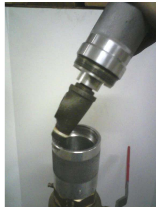
Unscrew and lift tee into the stuffing box and close valve. Tee removed.
