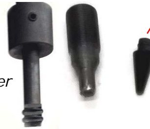
Remove punch, then insert Self Tapping Plug into main
