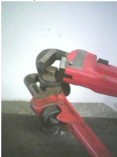
Plug tighter than tee
