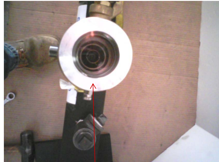
Over head view of sight glass attachment.
