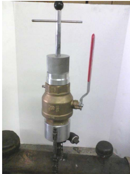
With the valve open push the plug adapter down onto the square head of the plug. Unscrew plug and retract it above the ball valve. Close valve.
