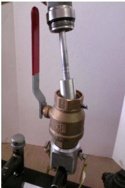
Plug adapter with integrated magnet.
