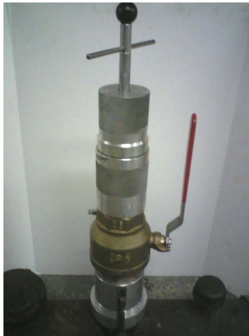
Open valve and push down on plug removal shaft locating it onto the plug square.
