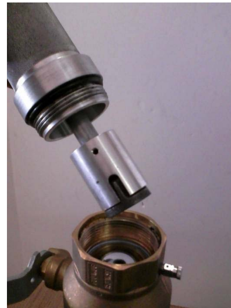
Pull up the handle to remove the cap and close the ball valve. The cap is held secure with an imbedded magnet.
