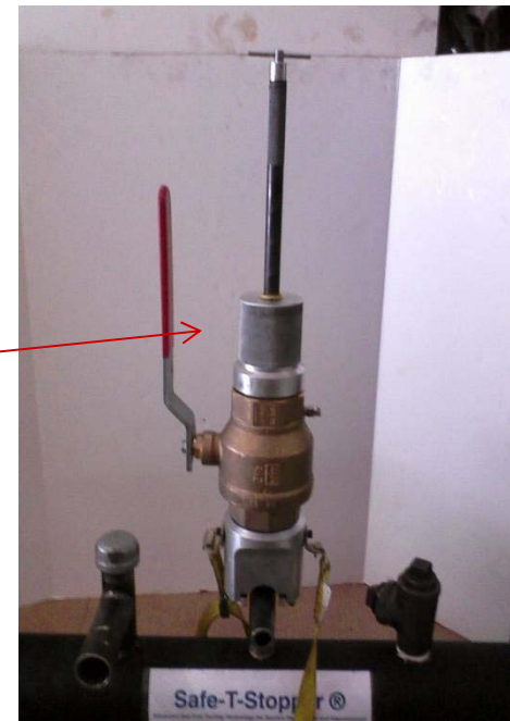
Expansion stopper inserted and expanded below the branch stopping off the flow of gas. The cap is replaced and the service line cut and terminated.
