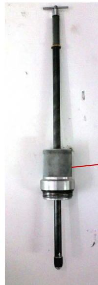
Expansion stopper tool (Inserts and removes expansion plug).
