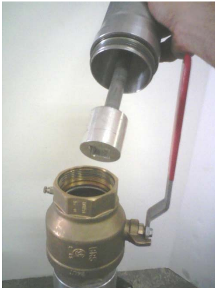
Plug adapter with integrated magnet.
