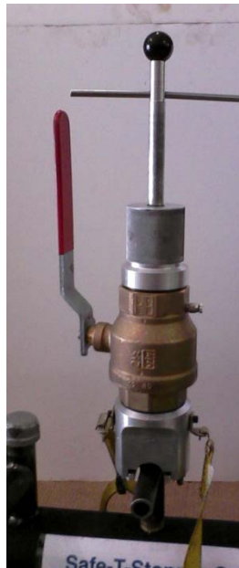
Attach and lower the adapter onto the cap. Rotate the handle counterclockwise loosening the cap.
