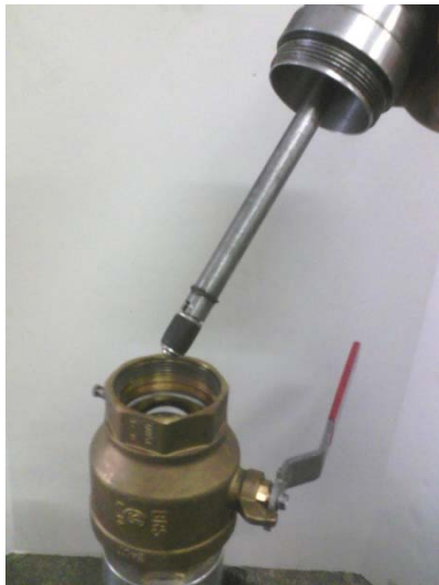
Expansion plug insertion tool
