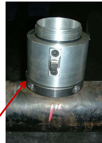
Base adapter: Half collars that seal around coupling.
