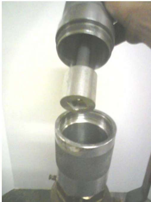
Magnetic plug removal adapter.
