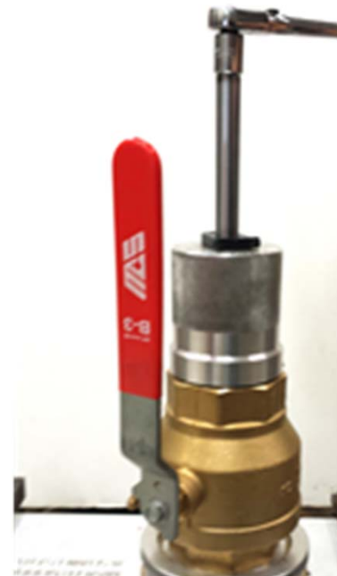
Push down and tighten plug into main to stop the flow of gas.
