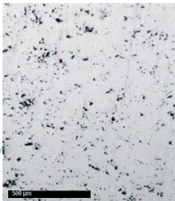
Fig. 1: Porosity of a P/M steel sample after a 4 min. polish with 3 µm diamond
