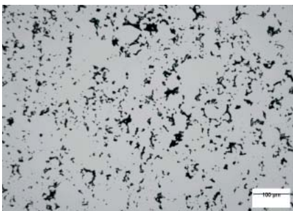
Fig. 8: Same sample as in Fig. 7 after longer polish showing correct porosity
