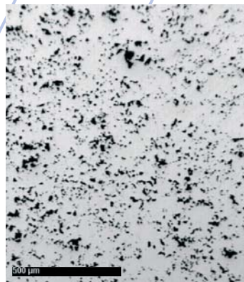
Fig. 2: Same sample as Fig.1 after 8 min. polish with 3 µm diamond
