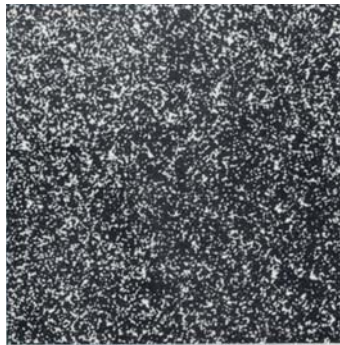
Fig. 5: Carbide distribution in powder metallurgically produced steel
