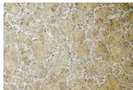
1018 Water Quenched steel, 400X (B.F.), etched with 2% nital, Structure is Bainite
