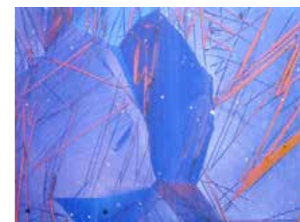
Fe-Ni-Co-Al Alloy, 400X (Polarized Light)
