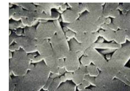
SiAlON ceramic, etched in molten KOH, Mag 20 KX
