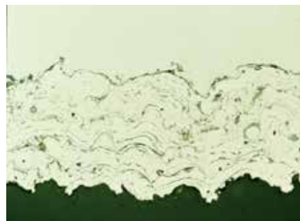
Nickel Chrome Thermal Spray Coating, as polished, Mag 1000x (B.F.)
