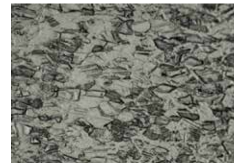
99.9% Silver, etched with ammonia peroxide, 200X B.F.
