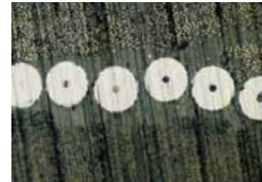
Boron-graphite composite sectioned with fine grit diamond wafering blade. Boron fibers damage minimal
