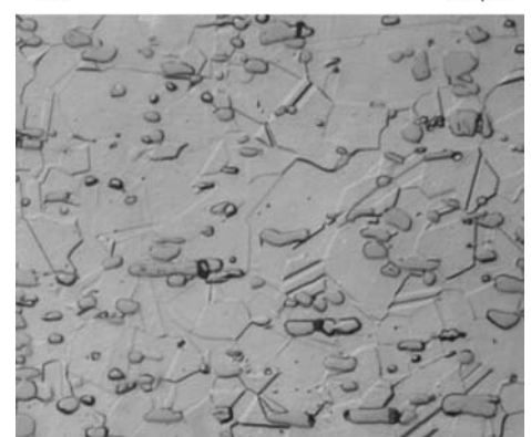
Fig. 37 The microstructure of 304 stainless steel plus boron enriched in the B^{10} isotope for nuclear reactors (Nautilus-class submarines). (a) Etched with waterless Kalling's reagent. (b) Etched with waterless Kalling's reagent but heavier than (a) to reveal the grain boundaries
